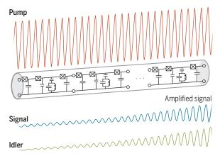
a transmission line. In a sense, the single motor on a swing is replaced by a series of motors on swings, where the motor-driven swings are linked together so that the motion of one swing is passed to its neighbor, and each motor slightly amplifies the motion as it is passed along the chain. This reduces the demand on each motor.
